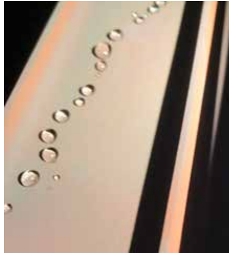
Figure 2: hydrophobic film on the deaerator trays
