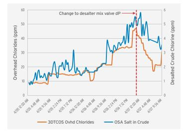
The online analyzers alerted the Operations Team to these increases and it was quickly determined that the reduction in feed rate caused a reduction in the mix valve dP, impacting desalting efficiency.
