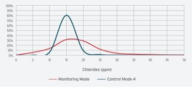
90% within the specification limit of 20ppm, was in fact only 80% compliant with a high degree of variability.
