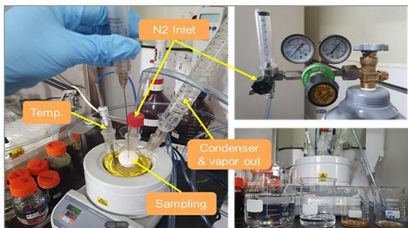
Figure 2: Shutdown Polymer Risk Assessment Test Equipment
