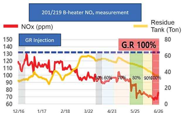
Figure 4: NOx reduction trend due to use of Green Retarder conversion residual fuel - 1.
